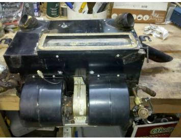
With the heater box out of the car, you can clean all the area back there, reroute accessory and stereo wire, and even fix any rust that may reside around the fresh air vent.
